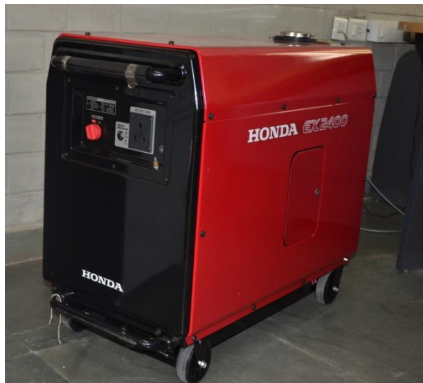
2.4 KVA portable generator set matter
